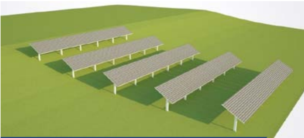
Figure 1B: Tracker Table Shadows on Variable Sloped Ground (Note the length of the shadow cast by the tables is shorter for tables on the slope)
