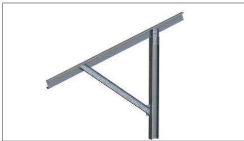
Articulating purlin connections combine with telescoping post bracket to navigate up to 15% terrain slopes
